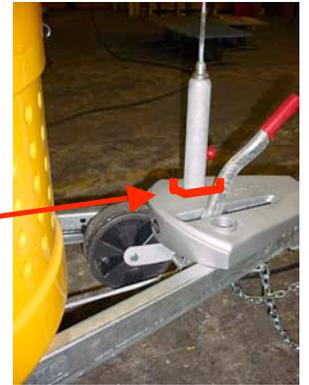
(Fig. 3) Jack/Wheel in up position
