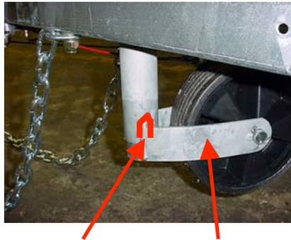
(Fig. 2) Notch; Dolly Wheel support arm
