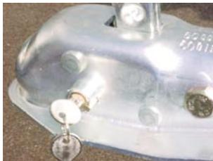
T@B trailers include a coupler lock to prevent theft. To Use, simply insert the key and lock into the opening on the side of the coupler. Turn key and remove. The coupler is now locked. The lock can be used whether the T@B is attached to your hitch.
