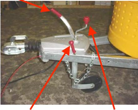
(Fig. 1) Quick release lever; Top-wind jack
